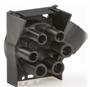
3. Powder-based. Powder is selectively bound together. SLS (Selective laser sintering). Is the rapid prototyping technology of choice for a range of functional prototype applications, including those with snap fits, living hinges and other mechanical joints. The most employed materials on SLS prototyping are PA, PA-GF, Rigid GF, PEEK, PS, alumide, carbonmide and elastomers.
