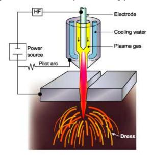
In plasma cutting there are two principal working systems, hand-held and computer numerically controlled (CNC). Hand-held is used up to 38 mm for fast and less accuracy cuts. Secondly CNC systems are used to make precise incisions up to 150 mm thick.
