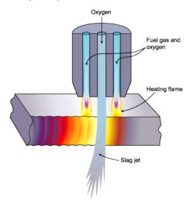
This process has a lower edge quality than waterjet or laser, but oxyfuel low-cost equipment and the cutting speed made this operation competitive. Equipment can be used manually or mechanised.
