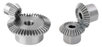
• **Spiral bevel gear:** This type of gear consists on a bevel gear with a helical angle of spiral teeth. Spiral bevel gears have the same advantages and disadvantages relative to their straight-cut cousins as helical gears do to spur gears. It is much more complex to manufacture, but offers a higher strength and lower noise.
