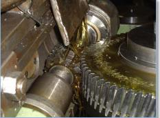
Ours factories can produce gears by several process, it could be with stock removal, like, for example: Gashing and hobbing, milling, broaching, gear shaping, etc. or without stock removal such as: sand casting, injection, stamping, extrusion and powder metallurgy. Thus as finishing operation and surface treatments like nitriding and carburizing including grinding, honing and lapping.
