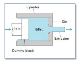
Many cross sections are manufactured by this method. The cross section produced will be uniform over the entire length of the metal extrusion.
