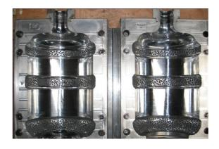
Blow molds are transported by corresponding mechanism into blow molding machines. Blow molding machines are formed by the blow mold, a heating and cooling system, which is necessary for its proper functioning, and an exhaust system that brings the piece to the outside when it is already in a solid state and a stable temperature. The exhaust system must have certain specific characteristics, such as design and power in order to no damage the piece.
