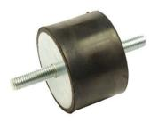
Silentblock bushing is a type of rubber bonded to metal isolator. These absorbers are able to remove or reduce a large amount of vibration problems, specialty when vibrations are of small amplitude.
